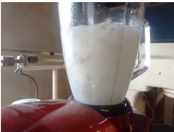
High speed mixing to destroy lumps
