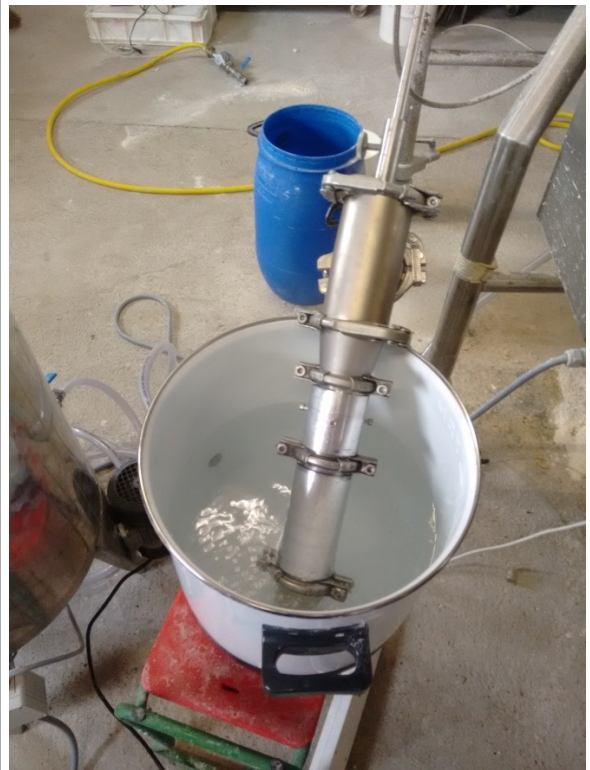
Heating up of equipment by pumping hot water in a loop
