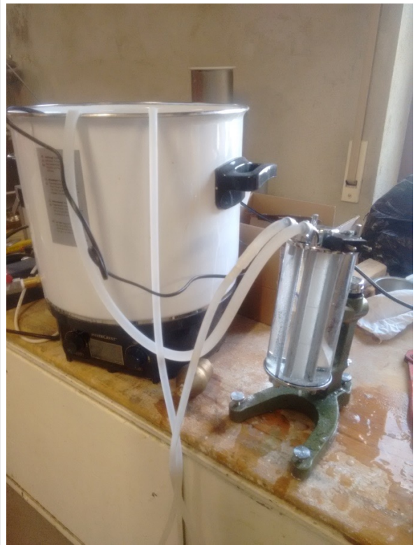
Water bath controlled setup at 27 °C
