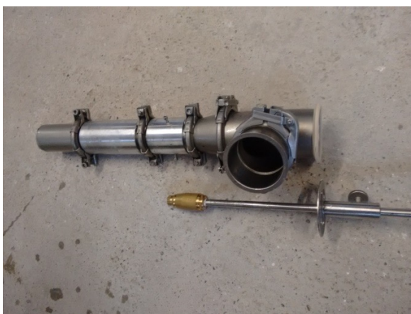
Mixing chamber disassembled
