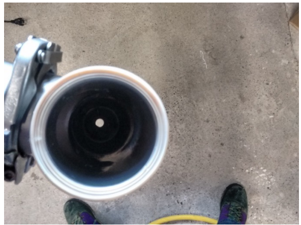
Look through mixing chamber with 1,5 cm diameter right under nozzle position
