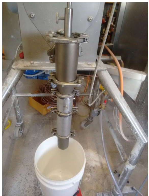
Rapidojet setup with "hydrocolloid" mixing chamber
