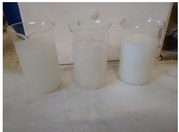
From left to right: Rapidojet mixed – handmixed with lumps – high speed mixed
