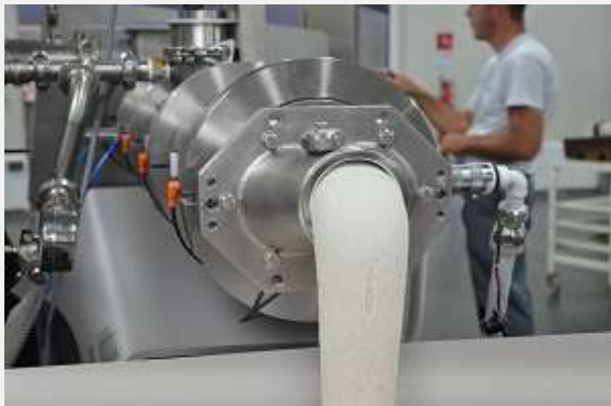
Continuous mixing under vacuum extends the shelf life of some products, according to mixing specialist VMI. The system was designed with the sponge-and-dough process in mind. Photo: VMI North America
