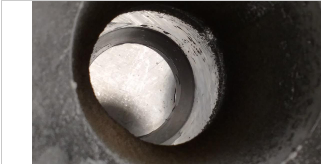
No residues on mixing chamber wall at cold hydration of pectin
