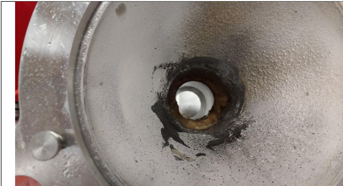
Some residues on the mixing chamber at hot water hydration of pectin
