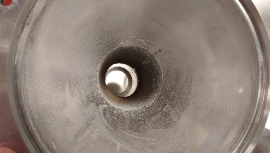
Mixing chamber: wet mixing area; no possibility for lumps to sit on the wall
